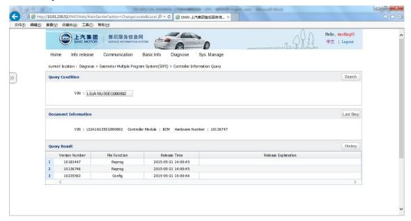
Step 6: Click "History", the pop-up box display software information released previously. The files with same "Module ID" indicate the software of same category. Distinguish different versions by "Version Number". Distinguish replacement relations by "Release Time". The one of the latest time is the new version.
