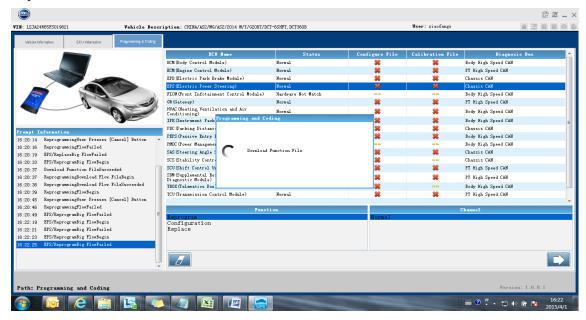
Step 3: Display the using data file information of EPS Reprogram function. "Vehicle ECU Information" indicates the information of current calibration version. "Manufacturer Database Information" indicates the information of currently available calibration version in the database (viz. calibration information to be written into the ECU). Through matching status, you may see the files needed for upgrading: "ECU Application Software", "ECU Calibration Software", and "Network Configuration File".
