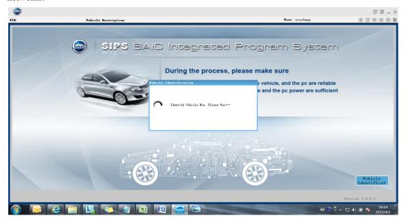
Step 6: Display vehicle identification results which will be used to carry out subsequent operations. Information displayed includes: VIN, mileage, model year, model, engine model and transmission model.
