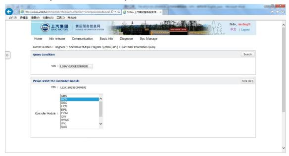
Step 4: "Hardware Number" lists the supporting hardware list of selected controller. Please select the hardware number of controller installed on the vehicle. Click "Next Step". To re-select controller, please click "Last Step";
