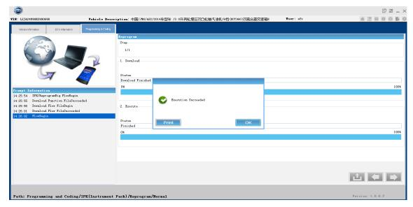
Step 9: Display Reprogram function execution results (succeeded) and list the execution result of each operating flow. Click "OK" to finish the function. SIPS goes back to "Programming and Coding" main interface and automatically refreshes EPS displaying information in the ECU list.
