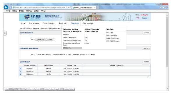
Step 2: This interface displays relevant user manuals and bulletins of SIPS system. Input corresponding query conditions (query conditions could be blank). Click "Search". After clicking on corresponding file, "Browse" may view and download files.
