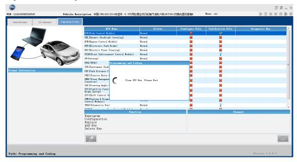
Step 4: Clear DTC succeeded. Click "OK" to go back to the "Programming and Coding" main interface.
