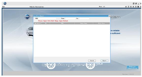
Step 2: Input at least one VIN query condition or time. Click "Search" and list the log files conforming to the conditions.
