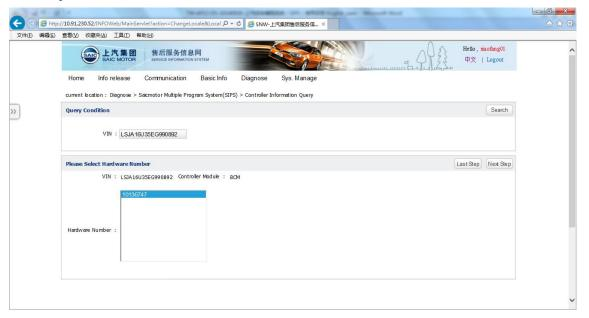
Step 5: Display corresponding latest calibration software information of selected controller and hardware. Each version of software may consist of several files. The interface lists version number, file function, release time and release explanation of all files contained in the latest version of software. Click "History" and you may view the information of version released previously.
